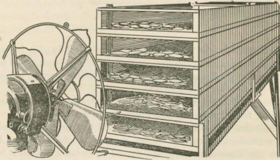
Drying by means of an electric fan.
