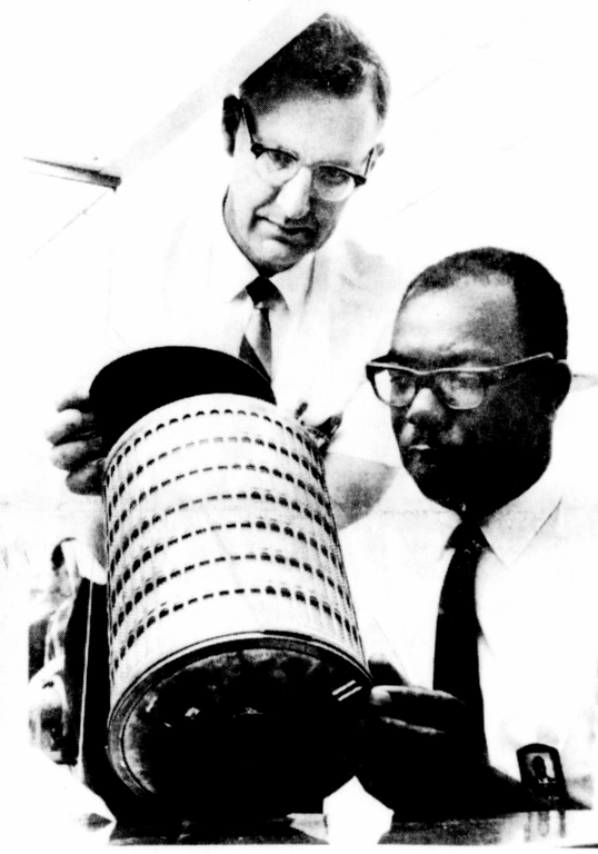
BACK FROM MOON — A lithium hydroxide cartridge used aboard Apollo 10 lunar module, which flew within 50,000 feet of the moon (rep. to recent successful landing of Apollo 11), is being examined by Ted Hammes of Enfield (left) assistant project engineer, and engineer Bill Ross (right), of Hamilton Standard. The canister, which removes carbon dioxide from the LM cabin air, was part of the craft's atmosphere revitalization package built by the local plant, and was brought back for performance evaluation.
