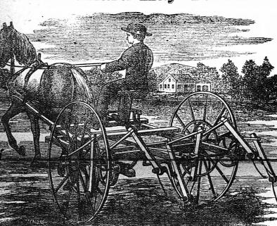
The only Tedder with forks outside the wheels, consequently the only Tedder that in passing back and forth the wheels do not pass over the tedded hay. More in use than of all other kinds together, the only Tedder that has stood the test of time
