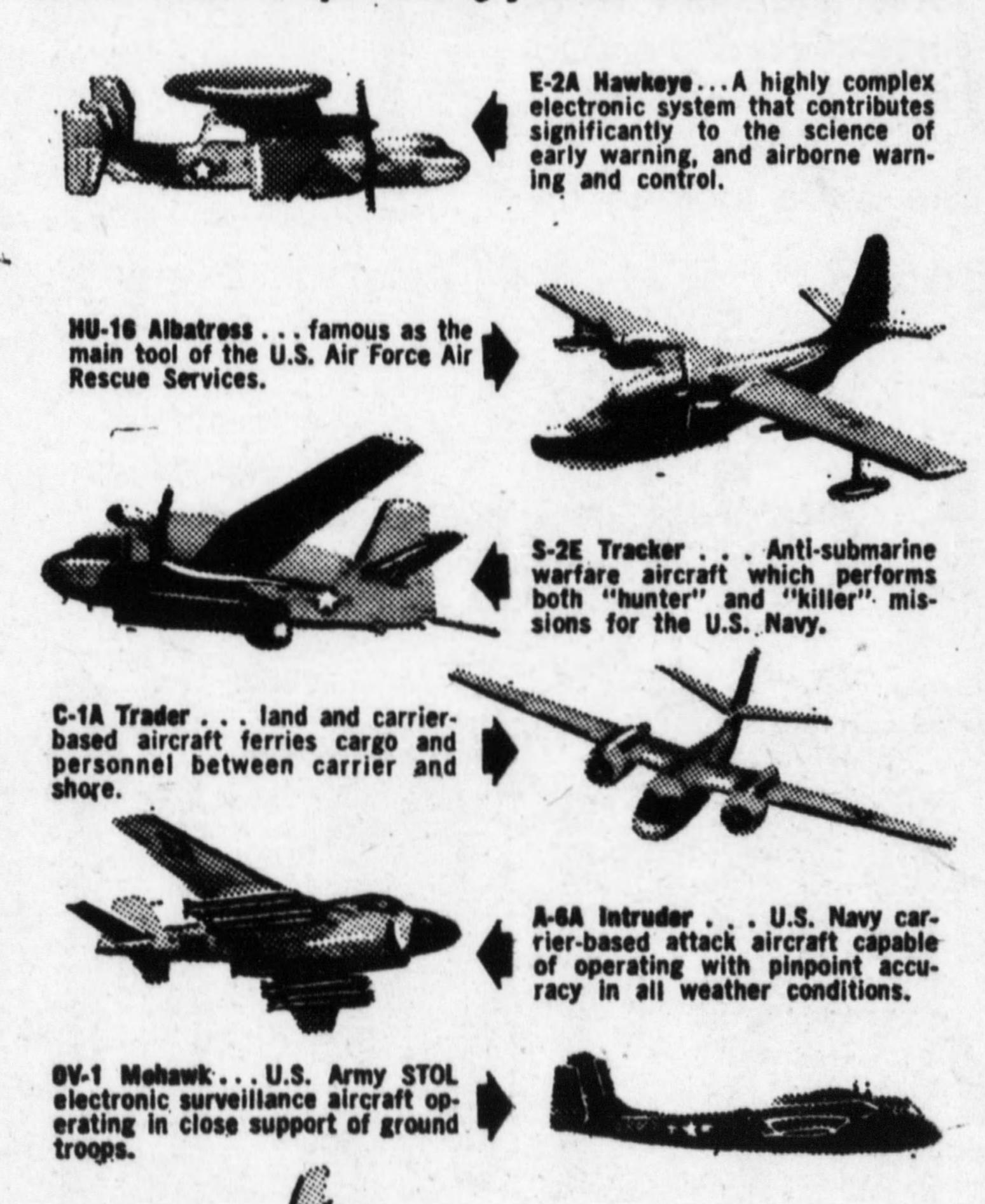
Currently, Grumman engineers, pulling the state of the art relentless forward, are engrossed in still more advanced aircraft and aerospace vehicles. These include:
